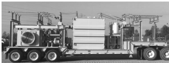
Modular Integrated Transportable Substation.
